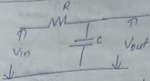
In a low pass RC circuit, the output is taken across a capacitor. Resistor offers fixed opposition. Since reactance offered by capacitor  $C$  falls with the increase in frequency, low frequency signal develops across the capacitor but signal of frequency above cut off  $f_2$  develops negligible voltage across capacitor  $C$ .
