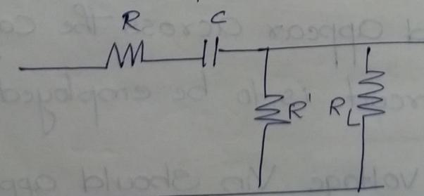
The time constant  $Rc$  of the circuit should be much smaller than the time period of the input signal  $Rc \ll T$
