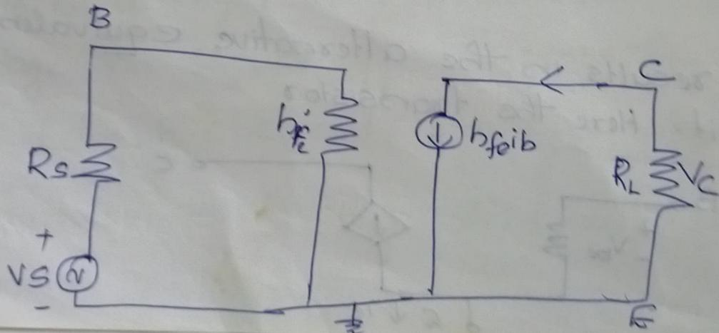
On the output side the resistance  $\frac{1}{h_{oe}}$  appears in parallel with the load resistance  $R_L$ . Under this condition, the magnitude of voltage of generator in emitted circuit  $b_{fe} V_C = h_{oe} I_C R_L = b_{fe} b_{fe} I_b R_L$ .
