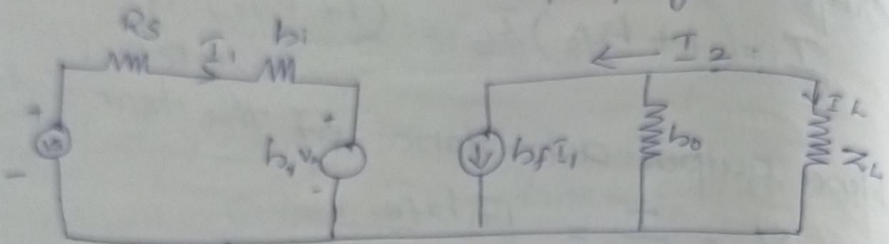
$A_I$  is defined as the ratio of output to input currents
